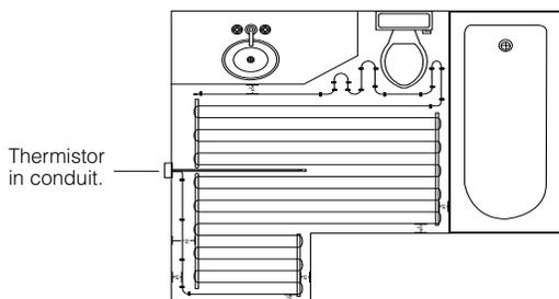
**Detail 2.** Install thermistor between two cable runs.
