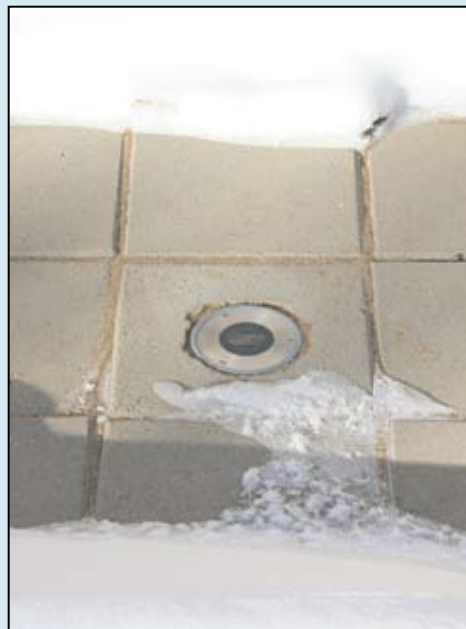
Snow Sensor Test Pad sensing snow and beginning to melt the snow.
