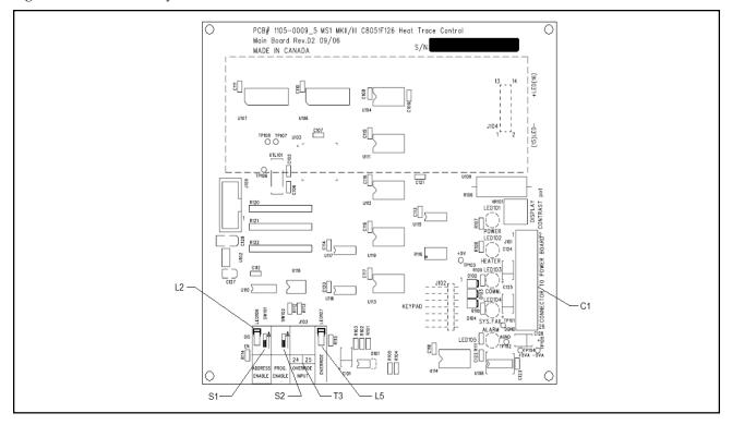
Figure 2.2 Power Board Layout
