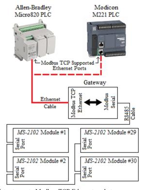
data stream to Modbus TCP Ethernet packets.
