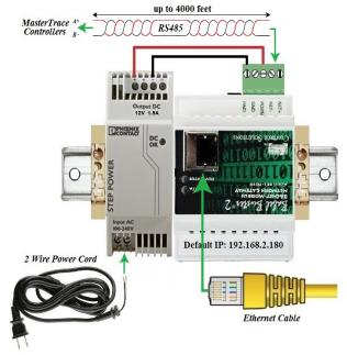
Configured MasterTrace Modbus to BACnet/IP Gateway
