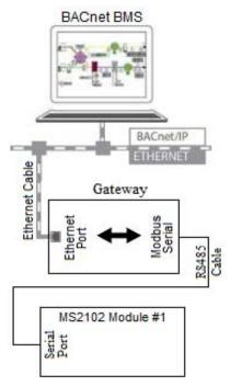
In a MS-2102 heat tracing control module with BAC
