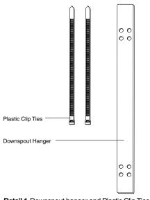
Detail 1. Downspout hanger and Plastic Clip Ties.
