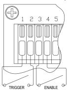
capability to trigger or disable the system through telephone or computer control. Closure of the Trigger and Enable inputs simulates the sensor MANUAL ON override. The sensor will remain in MANUAL ON as long as the inputs are closed. A momentary closure will trigger a snow melt cycle. Once the cycle is complete the sensor will revert to AUTOMATIC mode.
