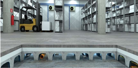
Illustration #11: Construction of a Ventilated Freezer Floor in a Cold Storage Facility.
