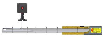
The trace heating system uses a parallel trace heater. Its fixed specific resistance offers a constant power output irrespective of the ambient temperature. The aluminum outer jacket ensures maximum mechanical strength.
