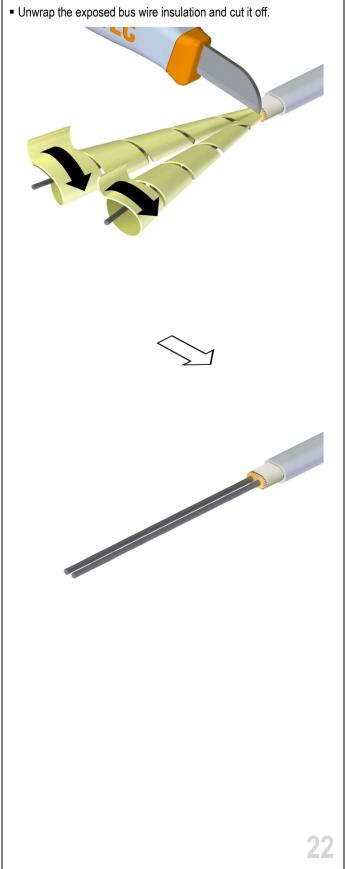
Make sure that all bus wires are intact and not nicked or damaged.
