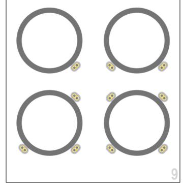
Fasten the trace heater on the pipe at intervals of a maximum of 18" (450 mm).
