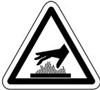
The outside surfaces of the heater are hot during operation and after operation. If contact is made, permanent skin damage may occur. Do not move, handle, or service the unit during operation or while hot.
