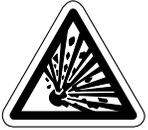
Failure to maintain minimum clearances to combustibles may result in fire and/or explosion, property damage, serious injury, or death. Always maintain minimum clearances and post signs or provided tags (F/N: LL001) adjacent to heater's controller. Signs should state the hazards for the particular application and be legible to the building occupants. Consult the factory or a factory representative for additional information on signage compliance.
