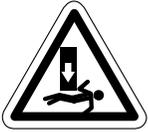
Improper suspension of the infrared heater may result in collapse and being crushed. Always suspend from a permanent part of the building structure that can support the total force and weight of the heater.
