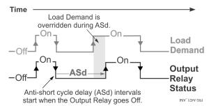
Anti-short cycle delay is typically used for refrigeration applications so that the system pressure can equalize before restarting the compressor.
