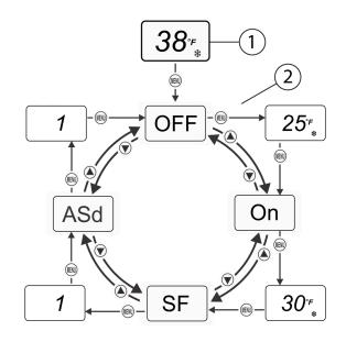
(i) **Note:** Use the **Up** and **Down** arrows to navigate through the basic menu, to return to the main screen and to edit settings in the menu. Press the **MENU** tab to save settings in the basic menu.
