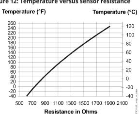
Figure 12: Temperature versus sensor resistance
