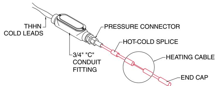
**Detail 1.** Dual conductor M.I. permafrost prevention heating cable assembly : Heating cable is typically installed in 1 1/4" rigid metal conduit below the insulation in concrete, asphalt or sand. The assembly is factory terminated and includes a base kit as described in section 1.2.
