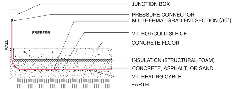
**Detail 9.** Side view of Installing M.I. cable in subgrade below thermal insulation.
