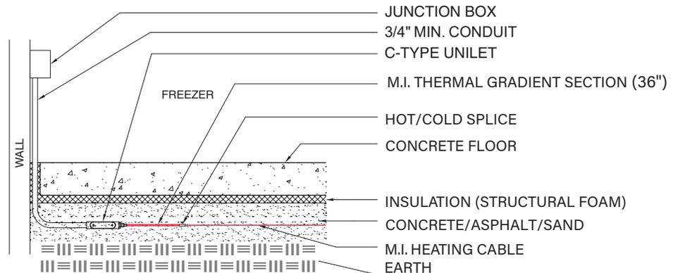
**Detail 8.** Side view of Installing conductor M.I. cable in subgrade below thermal insulation. M.I. cable is attached to a conduit system and conduit is attached to junction box.
