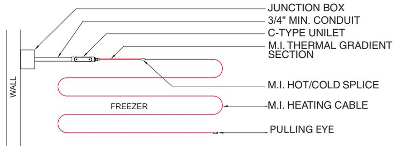
**Detail 6.** Plan view of Installing dual conductor M.I. cable in subgrade below thermal insulation.
