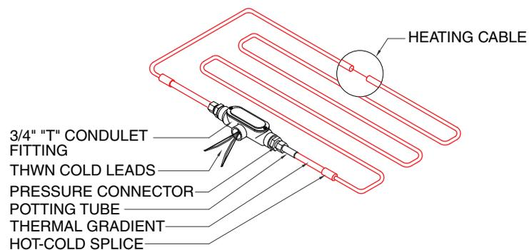
**Detail 2.** Single conductor M.I. permafrost prevention cable assembly is typically directly buried in the subsoil below the insulation. The assembly is factory terminated and ships with a base kit as described in section 1.2.
