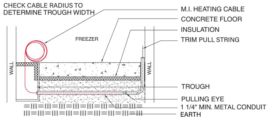
**Detail 4.** Dual conductor M.I. cable in conduit. M.I. cable is not being pulled through a 90° elbow.
