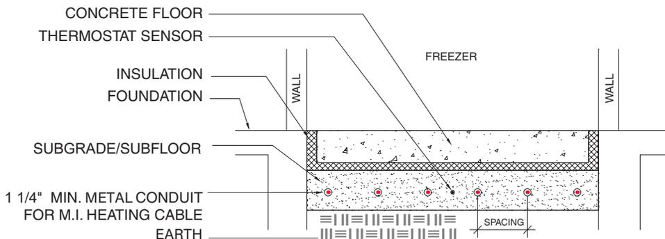
**Detail 5.** Install dual conductor M.I. cable and thermostat sensor in subgrade below thermal insulation.
