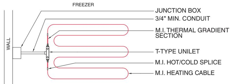
**Detail 7.** Plan view of Installing single conductor M.I. cable in subgrade below thermal insulation.
