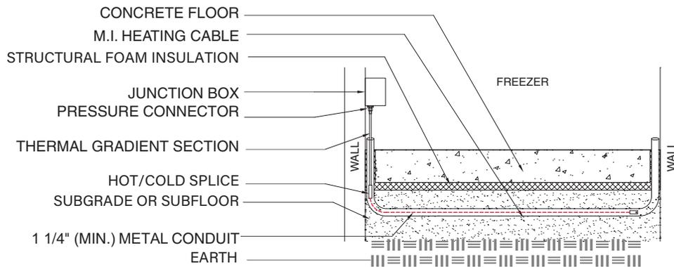
**Detail 3.** Dual conductor M.I. cable in conduit. M.I. cable is being pulled through a 90° elbow.
